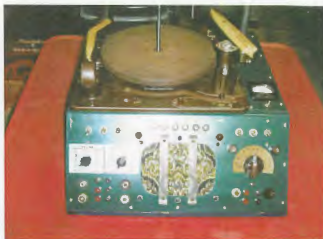
Vinyl record cutter and player, radio, PA system, and amplifier. I designed and built this combination unit in my senior year. There was nothing on the market like it until years later.
