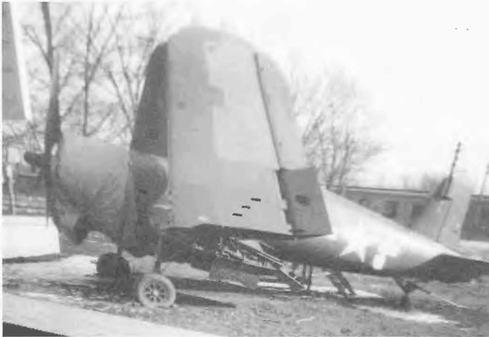
This photo shows the engine covered up with a canvas to protect it from the winter weather and spring rains. The plane was not all aluminum covered. Some areas were covered with fabric and it was starting to deteriorate.
